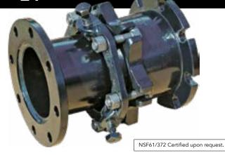
**NOTE:** Some initial axial movement may occur in lug style restraints as the lugs seat. Movement is directly related to the size of the piping system and the system pressure. In general terms movement of approximately 0.25 can be expected in restraints under 16". For larger sizes, movement of approximately 0.40 may be seen. If this is critical to your application please contact Romac Engineering for additional information.
