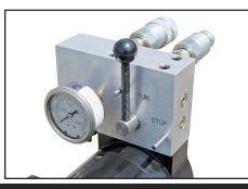
Integrated hydraulic drive head produces up to 15,000 inch lbs. of torque.
