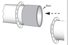
**Step 6** Clean and lubricate gaskets. Place the gasket without the tail on the insulating boot. Place the gasket with the tail on the opposite pipe, with beveled edge toward the pipe ends. If the coupling has two boots, then both will not have a tail, and can go on either side.
