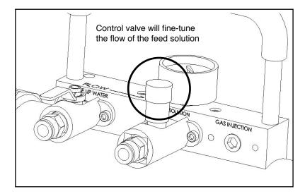
The feed solution flow can be fine-tuned with the control valve. This allows just enough dechlorinating solution to be fed to the water flow and extends the time between making up more batches of feed solution.
