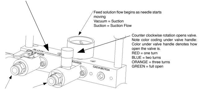
To install tubes on the Make Up Water Port and the Feed Soution Ports, just push tube in.
