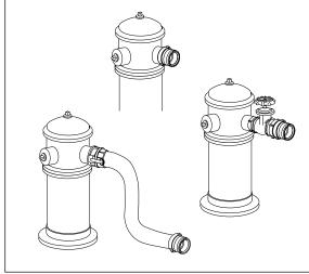
NOTE: When using deChlorinator at very high flows, be sure to place pin in hole (shown below) to prevent the camlock from blowing off.
