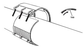
**Step 4** • Do not rotate the coupling or the pipe during tightening.
