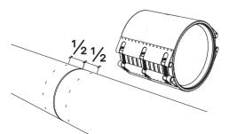
**Step 2** • Loosen the bolts with the o-rings until the clamp can be opened.
