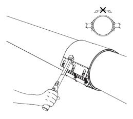
**Step 5** • If necessary, you may hydraulically test the clamp up to 1.5 times the working pressure shown on label.
