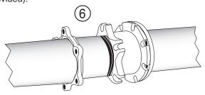
**Step 7** • The pipe should be centered such that the space between the OD of the pipe and the ID of the FCG is even all around the pipe. Slide the FCG gasket into position with the beveled edge engaging the beveled end of the FCG body.
