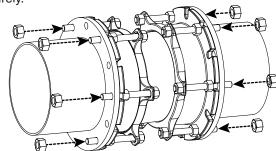
For 3" – 10" ECF400 sizes, tighten to 50 ft-lbs. For 12" ECF400 size, tighten to 90 ft-lbs.
