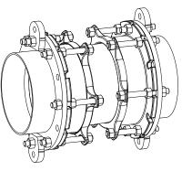
Step 8 • Install the tie rod through the harness lugs and place a set of spherical washers on the back side of each harness lug. Attach a nut at each end and tighten finger tight and then another 1/2 turn.
