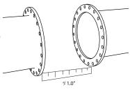
**Step 3** • Unpack the fitting. Loosen the end ring nuts on the thru-bolts to allow the spool piece to move freely within the flange coupling bodies. Remove the nuts that are on the flange face (O-Ring gasket seal is on this side). Place a mark at the center of the spool piece to make it easier to center the spool during assembly.
