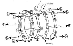
**Step 4** • Lift the ECF400 into position with the flanged coupling assemblies intact and fit the protruding thru-bolts into the corresponding flange bolt holes. On each flanged end, thread the nuts back on the thru-bolts and tighten securely.
