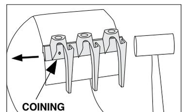
If your clamp has multiple lugs, tap the end lugs off first (see illustration). The lugs in the middle won't have coining and should slide off without using a hammer.
