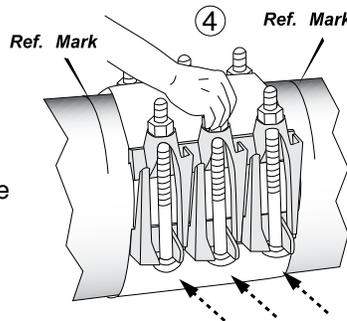
**NOTE:** If necessary (because of water pressure), Step 3 and Step 4 can be performed beside the pipe damage. Slide the clamp over the damage after the bolt heads have been snapped in place.
