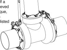
**Step 9** • Confirm proper installation by pressurizing the line and checking for leaks.
