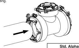
**Step 6** • Set the desired pipe deflection. **Note:** Do not deflect pipe joint after installation.
