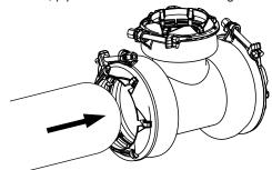
**Step 6** • Set the desired pipe deflection. **Note:** Do not deflect pipe joint after installation.
