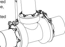
**Step 9** • Confirm proper installation by pressurizing the line and checking for leaks.
