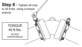
**NOTE:** Do not use an impact wrench. Do not overtorque, or retighten. If a good seal is not achieved at the installation torque, refer to the Common Installation Problem listed on side two.
