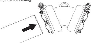
**Step 6** • Set the desired pipe deflection. **Note:** Do not deflect pipe joint after installation.
