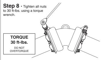
**NOTE:** Do not use an impact wrench. Do not overtorque, or retighten. If a good seal is not achieved at the installation torque, refer to the Common Installation Problem listed on side two.
