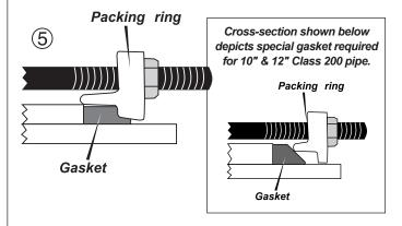
Step 6 Tighten bolts evenly around the pipe in 15 ft-lbs increments.
