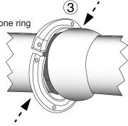
Step 4 • Assemble the other ring around the pipe behind the bell. Insert bolts and hand tighten all nuts.10" and 12" come with flat washers.
