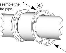
Step 5 • Make certain the gasket is under the packing ring as shown in the sketch.
