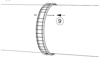
**Step 10** • Be certain that the center ring is started into the end ring, and is not interfering. If necessary, wedges can be used to free the end ring from the edge of the center ring.
