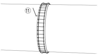
**Step 12** • After final torque has been achieved, remove all jacks and posts needed to round up the pipe.
