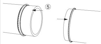
**Step 6** • Slide the center ring into position and center over the pipe ends. Slide gaskets into position with the beveled edge engaging the flared end of the center ring. Maintain the recommended gap between pipe ends as noted in the table below.
