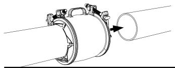
There should be a minimum of 6" of pipe insertion per coupling end. Confirm proper alignment between pipes and maintain the recommended minimum gap between pipe ends (1/4" - 1/2").
